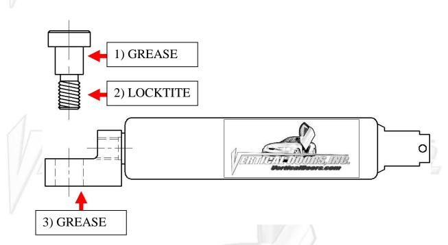
\*IMPORTANT STEP: DO NOT SKIP THIS STEP. THIS STEP IS CRUCIAL IN YOUR INSTALLATION PROCESS, IF THIS STEP IS NOT COMPLETED WHEN INSTALLING THE VERTICAL DOOR KIT; ALL WARRANTIES ARE VOIDED, AND MAY CAUSE FUTURE PROBLEMS WITH YOUR VERTICAL DOOR SYSTEM. 1<sup>ST</sup>, make sure you put grease on the body of shoulder bolt where the arrow is pointing.
