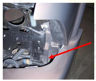
Remove all the 13mm bolts from the top of the fender and one bolt from the front of the fender by the headlights.
