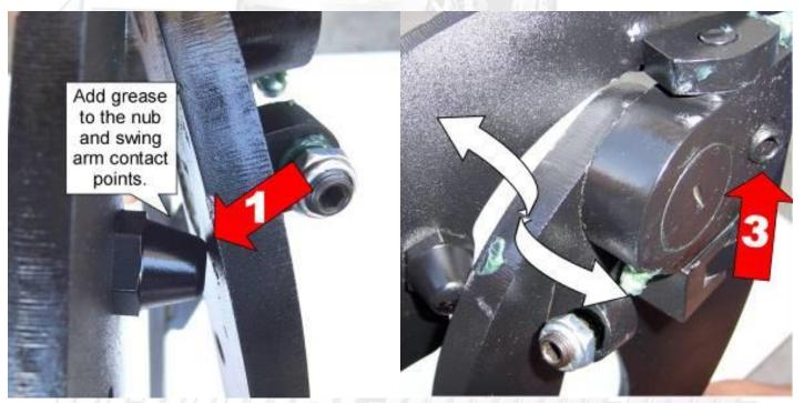
Hint\* (Fine tune the Allen Adjustment screw (#2) to realigned striker with door. After the door is align test door by opening and closing, lifting and lowering door several times.
